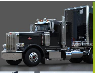
Adding a sleeper to an existing tractor can be impossible due to the swing clearance of your trailer. We have designed the DC-27 to give you as much room inside for a comfortable night's sleep without using up your valuable frame space. The DC-27's ultra light panel construction adds less than 200 lb. to your GVW.
