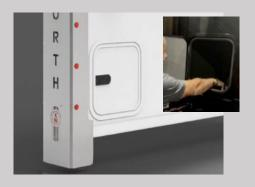
Back wall Access Doors Large 13" x 13" Located on the back wall Allow you to change out of your muddy boots and hang up your wet coat before you hop in the cab
